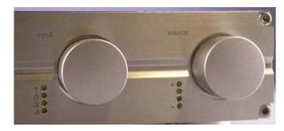
**Input Selection Knob** (left knob) – Push it in to turn P-8S On and Off. Turn the knob to select Input 1, 2, 3, or 4. If the P-8S is muted, pushing the Input Selection Knob once will bring P-8S out of muting.
